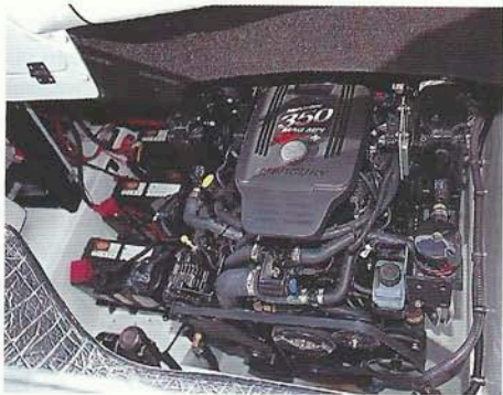
ABOVE: The review boat was fitted with a 300hp MerCruiser 5.7 litre V8/Bravo 3 sterndrive that proved a good combination for the new CR2800.
